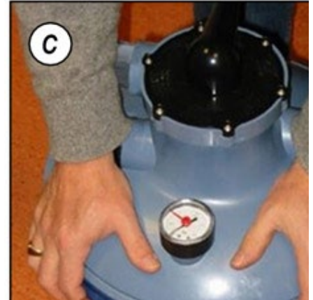
Position your two hands on the lid such that they are equidistant both from each other and your knee (120° angle)
