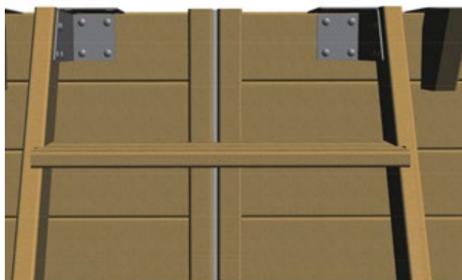
Figure 16 – Fastening the access ladder to the pool wall
